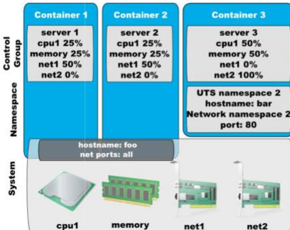
Figure 3 Container Components
