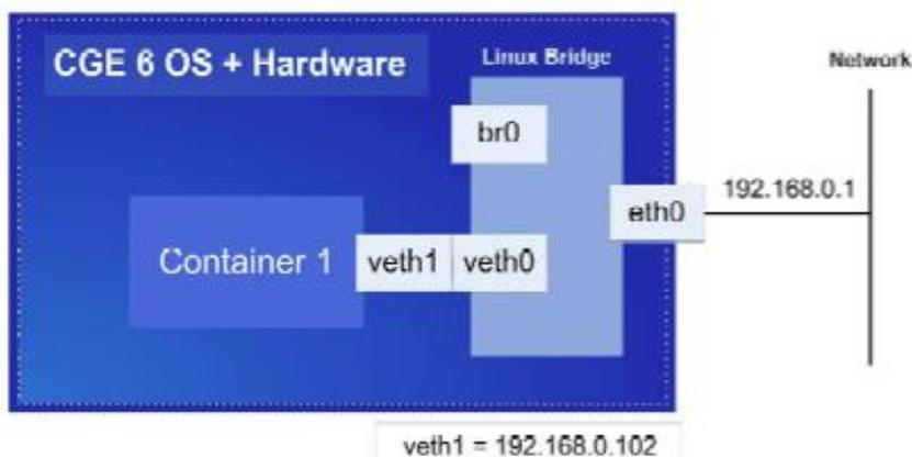
Figure 5 Configuring networking in a new network namespace
